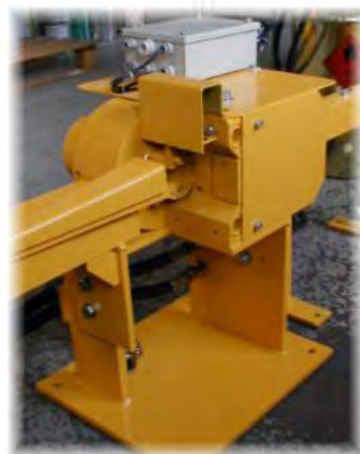
Hydraulic cutter 140 kN
